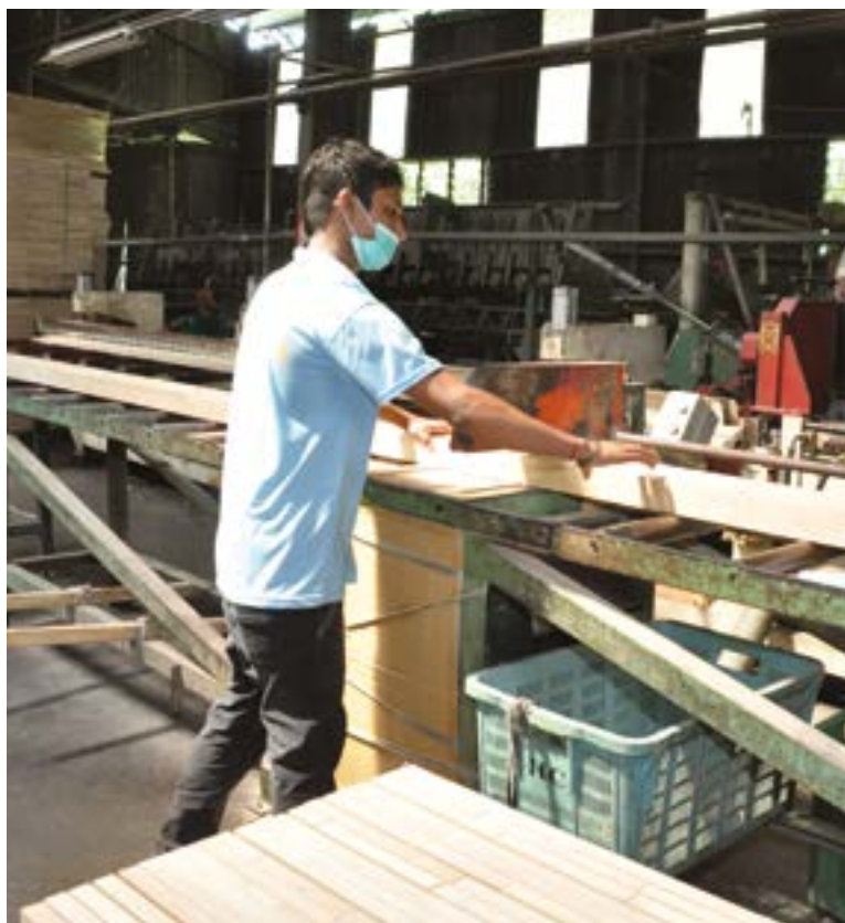
About 70% of Hup Chong's raw material is Rubberwood-based. The Rubberwood is finger-jointed and edge-glued, an efficient way to maximise yield.
