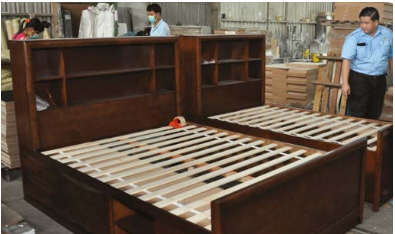
Quality assurance of its furniture products are performed at specific check-points by incoming material inspections, process QC and pre-shipment inspection.
